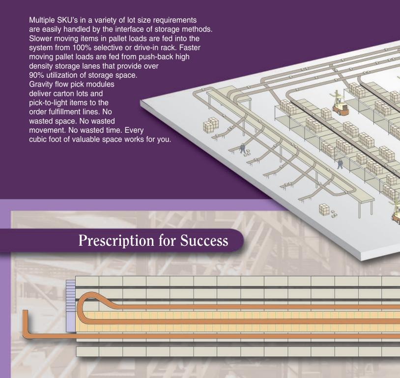
Ridg-U-Rak provides a multiple level, highly concentrated order picking system for one of the nations leading pharmaceutical manufacturers. Conveyors carry totes through upper level of
